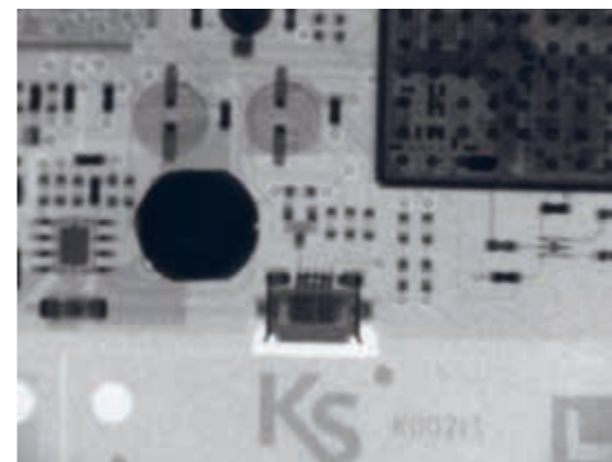
example of X-Rays Quality Control aiming to check soldering joints beneath the BGA Radio Module
